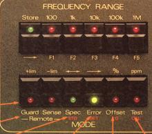
ERROR DEVIATION WITH  $\pm\,10\%$  ADJUSTMENT FOR DIRECT DISPLAY OF ACCURACY OF UNIT BEING CALIBRATED.
